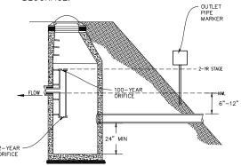
NATURALIZED DETENTION OUTLET CONTROL DETAIL
